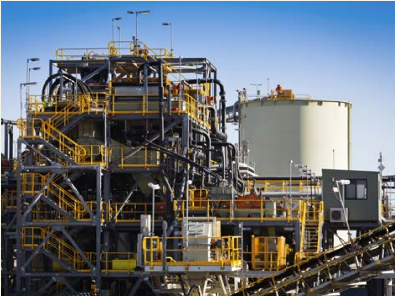
Mechanical processing used to refine lithium spodumene concentrate in western Australia. Lithium is used to produce high density batteries.
